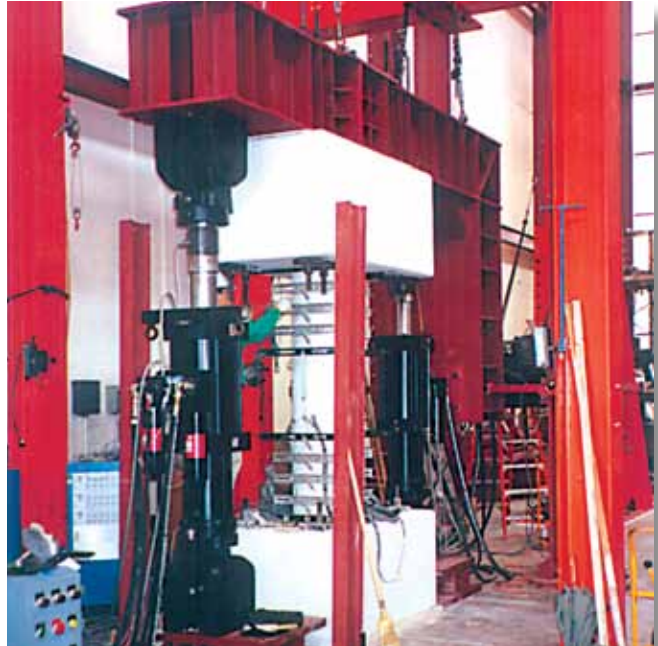
Dynamic Testing of a Column Support
