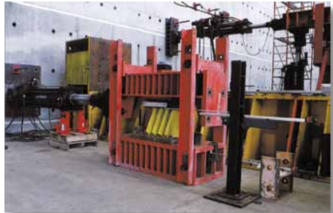
Substructure Pseudodynamic Test of TADAS device at NCEE
