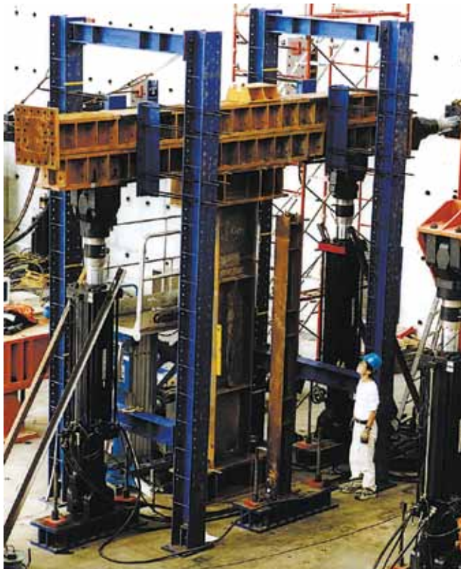
Substructural Pseudodynamic Test of DVF at NCREE
