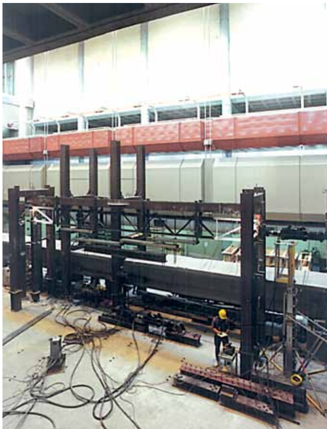
Quasi-Static Testing of a Bridge Structure
